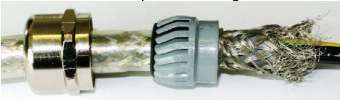
2. Place plastic bushing at 120mm, it should match up with the end of the end of plastic isolation of the cable.
