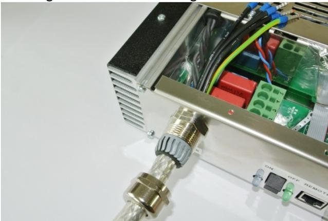
Pull the generator cable through the generator cable gland
