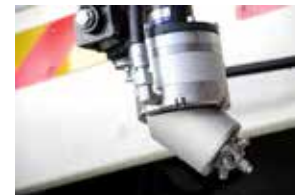
HTN bin washing nozzle washes whole bin in 15s run
